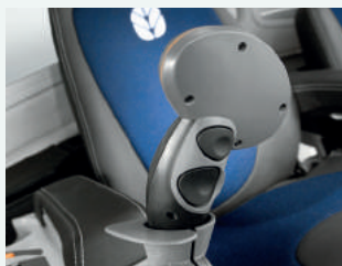
Shift button and ground speed unlock (behind).
