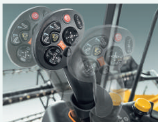
Force based movement enables the operator to change speed and direction.
