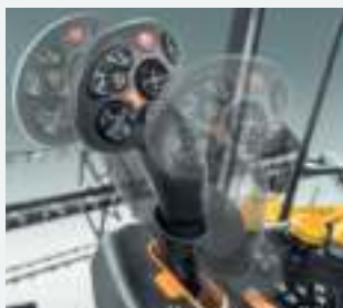
Force based movement enables the operator to change speed and direction.
